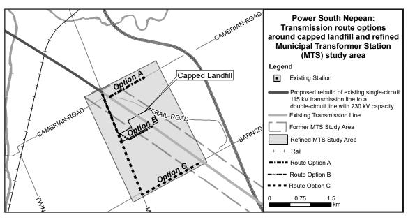
transformer station (MTS) and a new 230 kilovolt (kV) transmission line to connect the MTS to Hydro One's existing 230 kV transmission system at West Hunt Club Road. To achieve the connection line, Hydro One proposed to rebuild its existing single circuit 115 kV transmission line (3 wires) on the existing transmission corridor to a double circuit line (6 wires) with 230 kV capacity.
